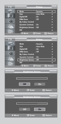
Brightness Sensor is to adjust brightness of screen either automatically or manually by detecting brightness of surrounding environment using light detecting sensor.
